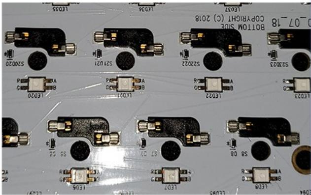
Top of PCB View Switches go on Sockets
